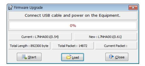
4) "Total Length" and "Total Packet" of the loaded firmware are displayed.
