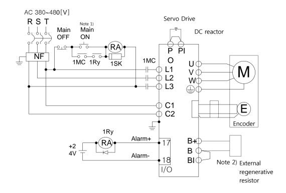
Note 1) It takes approximately one to two seconds until alarm signal is output after you turn on the main power. Accordingly, push and hold the main power ON switch for at least two seconds.
