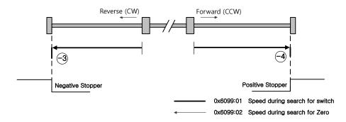
Homing method -3 and -4 only perform homing by using the Stopper. The velocity profile according to sequence is as follows. For more information, see the details below:
