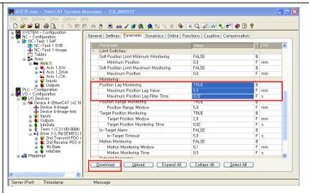
(Note) The Position Lag Monitoring is the difference between the position reference and the actual position at a given cycle time. When the Position Lag Monitoring is enabled, the TwinCAT NC generates an alarm if the positional error exceeds the settings.
