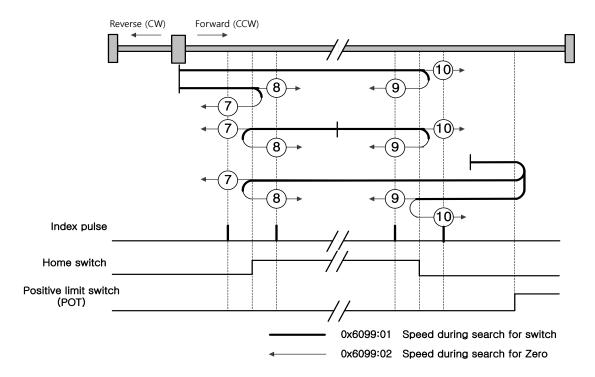
For homing using the Homing Method 7, the velocity profile according to the sequence is as follows. The sequence depends on the relationship between the load position and the Home switch at homing, which is categorized into three cases as below. For more information, see the details below:
