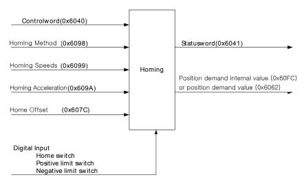
As shown in the figure below, you can set the offset between the home position and the zero position of the machine using the home offset. The zero position indicates a point whose Actual Position Value (0x6064) is zero (0).
