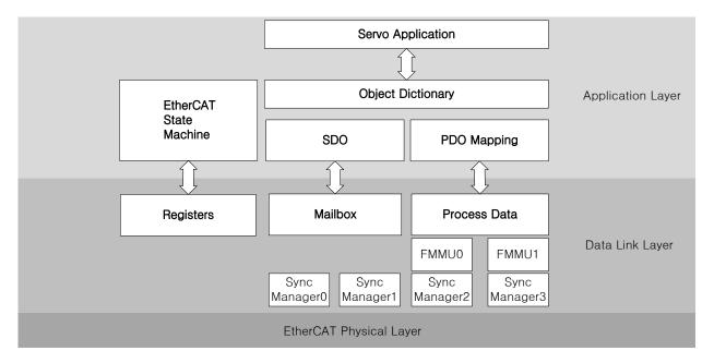
This drive supports a CiA 402 drive profile. The Object Dictionary in the application layer includes application data and PDO (Process Data Object) mapping information from the process data interface and application data.
