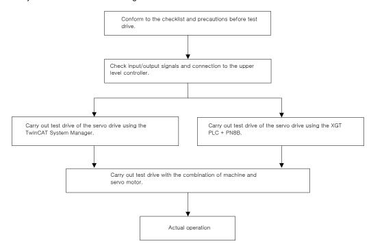
Verify that, before the test drive, the upper level controller and the servo drive are correctly wired, and the objects of the servo drive are correctly configured.
