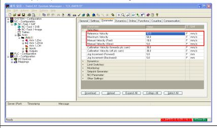
Set the speed, acceleration, and jerk of the test drive axis.
