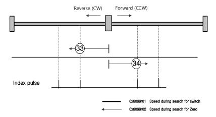
The initial driving direction is reverse (CW) for the method 33, and forward (CCW) for the method 34. The drive detects the index pulse at the Zero Search Speed.
