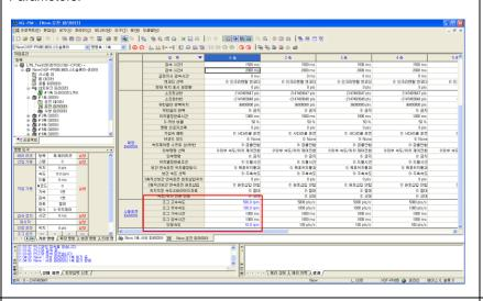
8 Set the servo parameters of the test drive axis.
