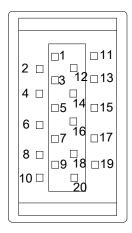
■ Analog Monitoring Connector Specification : DF-11-4DS-2C (HIROSE)
