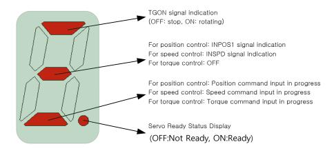
Digit5 indicates the status of the EtherCAT State Machine or of the current control mode and servo ON.
