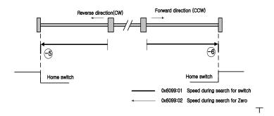
Homing Methods -5, -6 uses only Home switch to return to origin. The speed profile of each sequence is as follows. When limit switch is detected, Homing is stopped. Please see the explanations below for further details.
