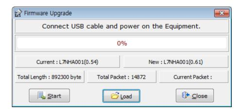
5) Press the "Start" button to start transmission. 10 seconds are counted down to clear the internal memory in the drive. (For L7NH and L7P, the segment 7 should display "USB". For PEGASUS, a red "ERR" LED should be illuminated.)
