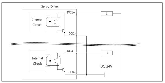
Note 1) For DO1~ DO4 output signals, the GND24 terminal is separated.
