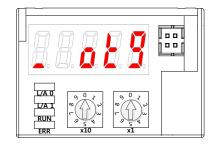
(7-segments display a message when downloading the firmware using the OTG)
