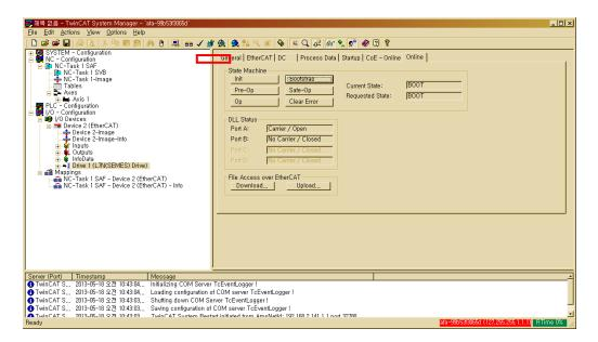
(3) After the current state is changed to BOOT and you check the drive status (7-segments display boot), wait for approx. 10 seconds until the internal flash memory of the drive is cleared.
