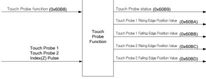
The position value of the encoder (Actual Position Value, 0x6064) is latched by the following trigger events according to the setting value. At the same time, 2 channel inputs can be latched independently at the positive/negative edges.
