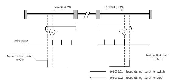
For homing using the Homing Method 1, the velocity profile according to the sequence is as follows. See the details below:
