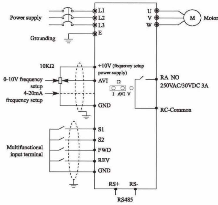
Note: AVI terminals can be used to select an analog voltage input(0-10V) and analog current input (4-20mA ) through the switch J2.
